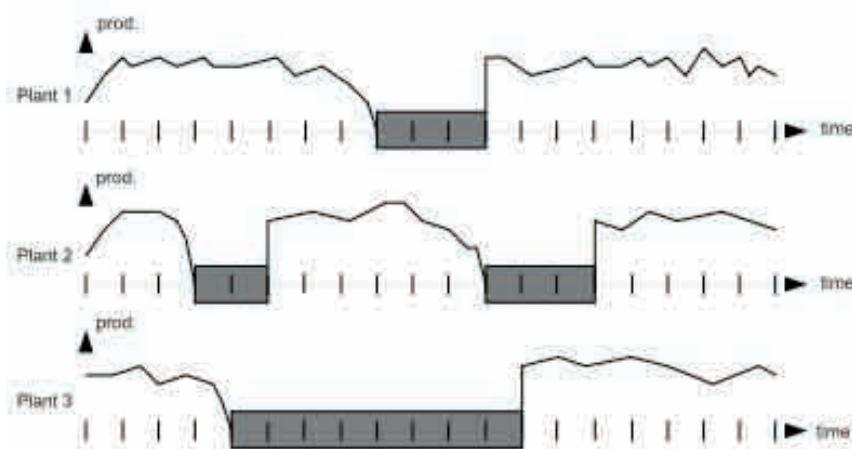
Figure 1: Outages, Cycles, Production Plans.
