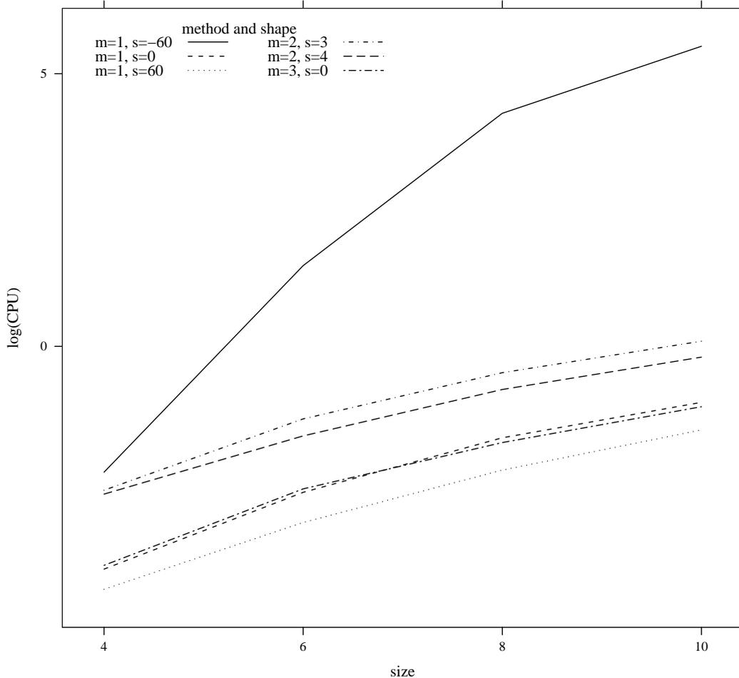
Figure 11: Logarithm of average CPU against  $n$  (cost range  $\{0, \dots, 10000\}$  and entry range  $\{10, \dots, 30\}$ ).
